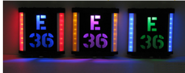
Patented firefighter's location signaling light (FLoSiL) Locating/Signaling System
