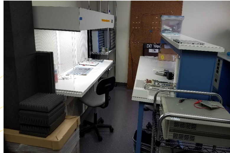
Clean Assembly Room - HEPA Laminar Air Flow
